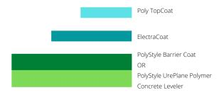
PolyStyle ESD must be applied by an authorized StaticStop Installer and is only sold as a turn-key, installed system. Concrete should be tested for moisture emissions prior to installation. Surface should be shot blast or ground to provide an ICRI profile of SCP3 or greater and all dust must be removed.
